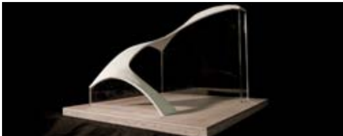
12 Final structure and TNA form finding result of the ETH Zurich Seminar Week Vault - 1:1 Thin-Tile Prototype.
