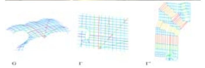
17 Final structure and TNA form finding result of the Pittet Artisans Vault - 1:1 Thin-Tile Floor System.
