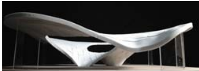
13 Final structure and TNA form finding result of the UT Sydney Ribbed Catalan Vault - 1:1 Thin-Tile Prototype.
