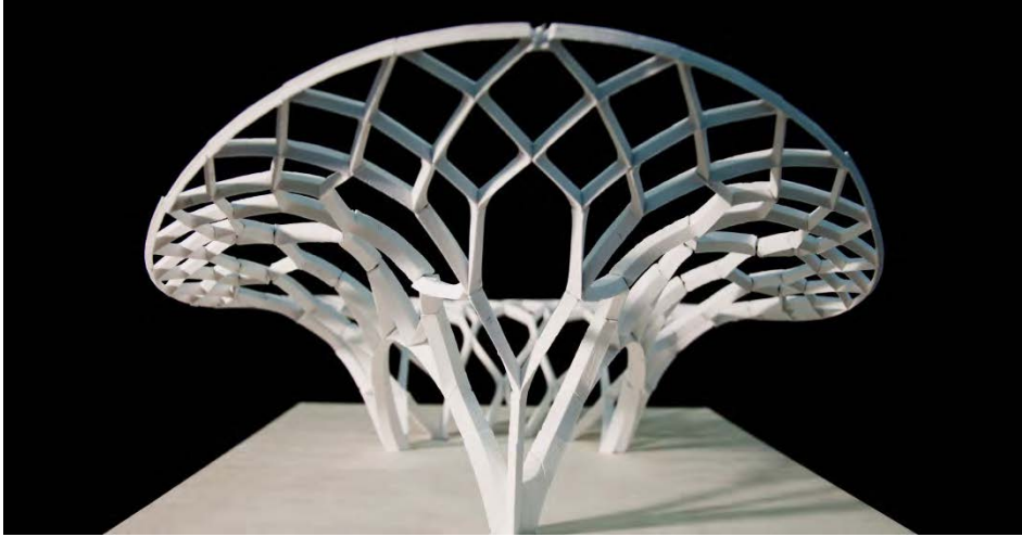
Figure 12: Structural scale model of a discrete funnel-shaped rib vault
