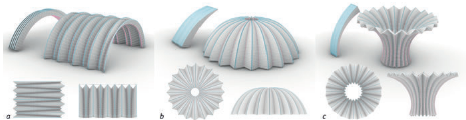
Fig. 12: Corrugated CCU (a) vault, (b) dome, and (c) funnel by plane inclination perpendicular to the actuation rotation axis.
