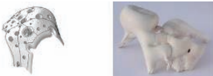
Figure 5: Fabric Form project shows considerable difference between digital model and latex and plaster model (Emery, et al. , 2011).
