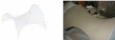
Figure 2: Physical prototype differed substantially from numerical model (Cauberg, 2009).
