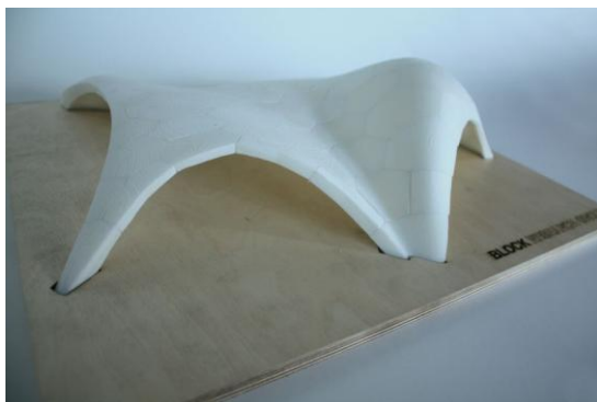
Fig. 8: Support details, showing the unglued pieces held together by compression.
