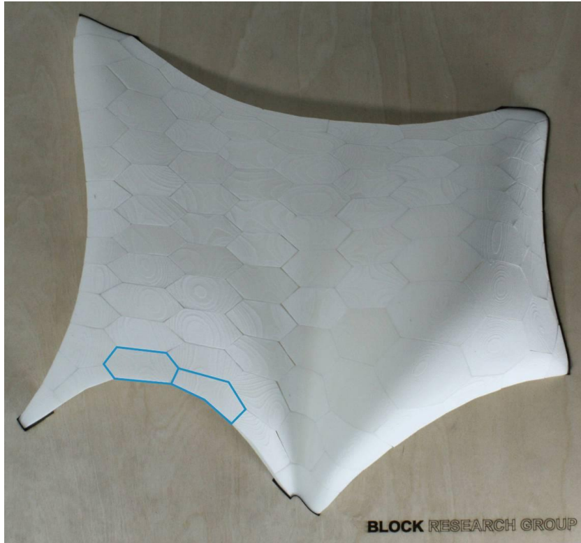
Fig. 7: Top view of the vault model with marked edge tessellation pattern.
