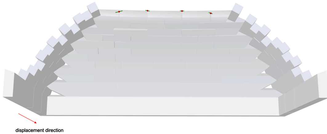
Fig. 18. Contact forces in the plane XZ. Contact forces in a horizontal row of the front web after seven displacement steps.
