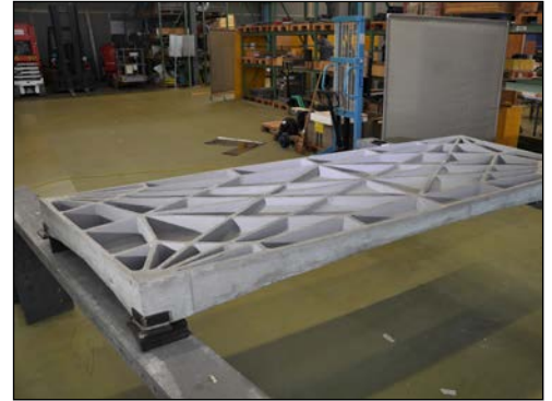
Prototype of the modular, vaulted, unreinforced concrete construction, no more than 2 cm thick.
