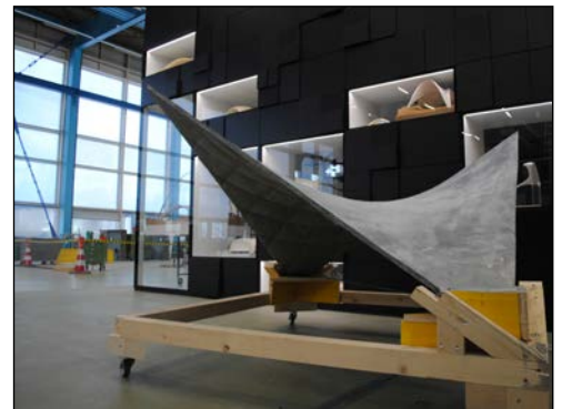
Prototype shell built using the new hybrid cable-net and fabric formwork.
